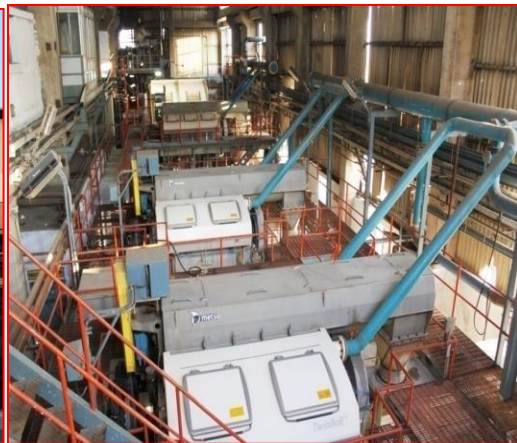
Twin Roll press for efficient pulp washing
